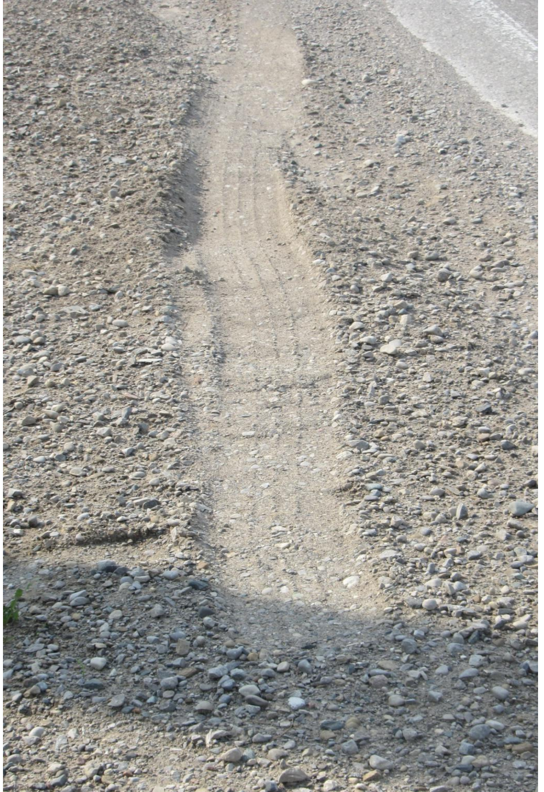
Figure 4: Southward view of tire mark caused by the left side tires of the vehicle.
