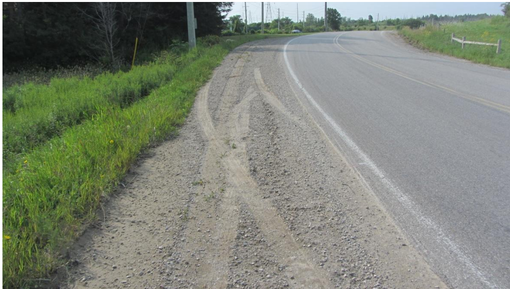
Figure 13: The tire marks terminate in the background where the vehicle stops its reversing and then accelerates forward toward the camera and back onto the road.
