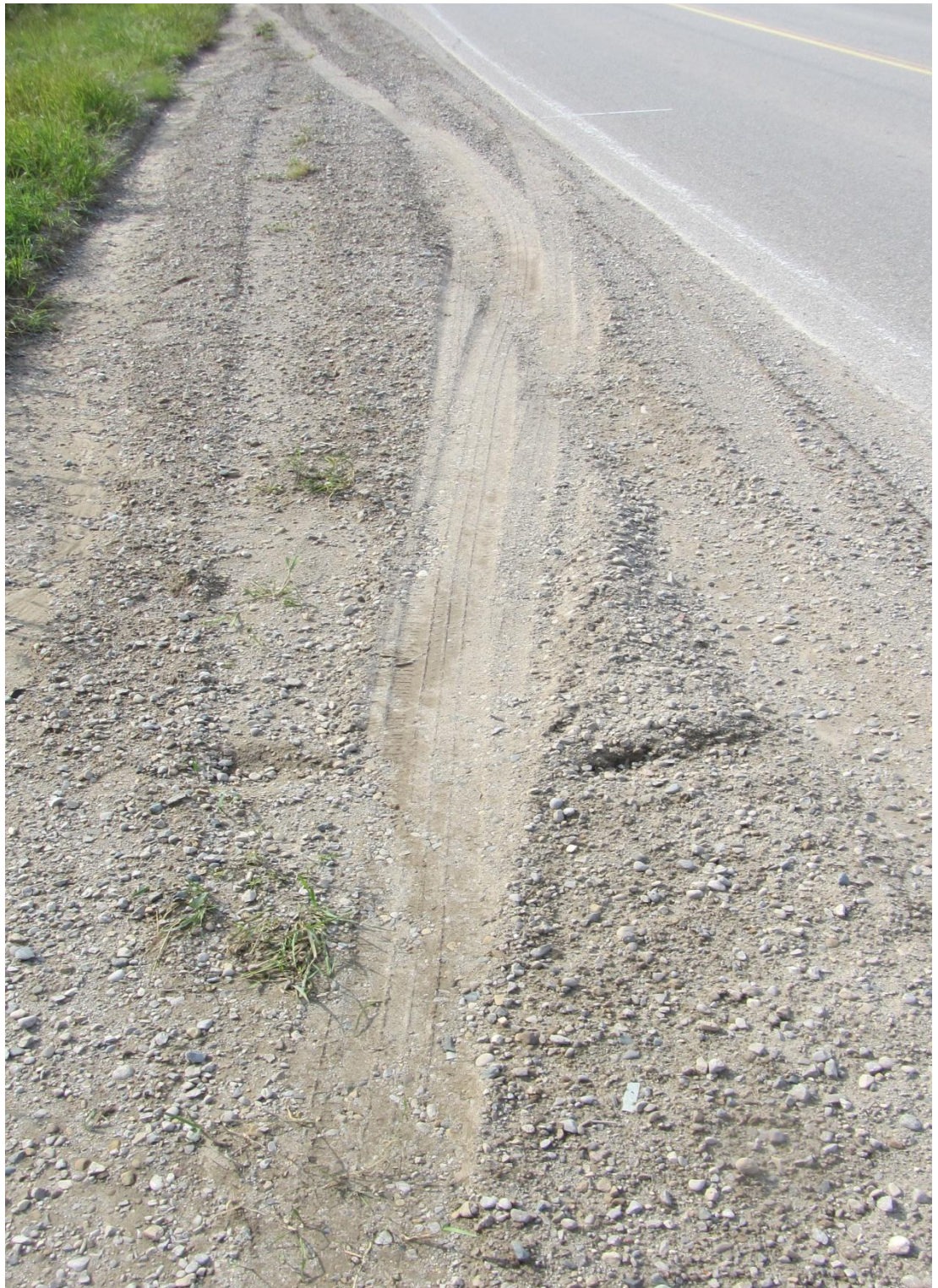
Figure 7: View of right tire mark as the vehicle reverses.
