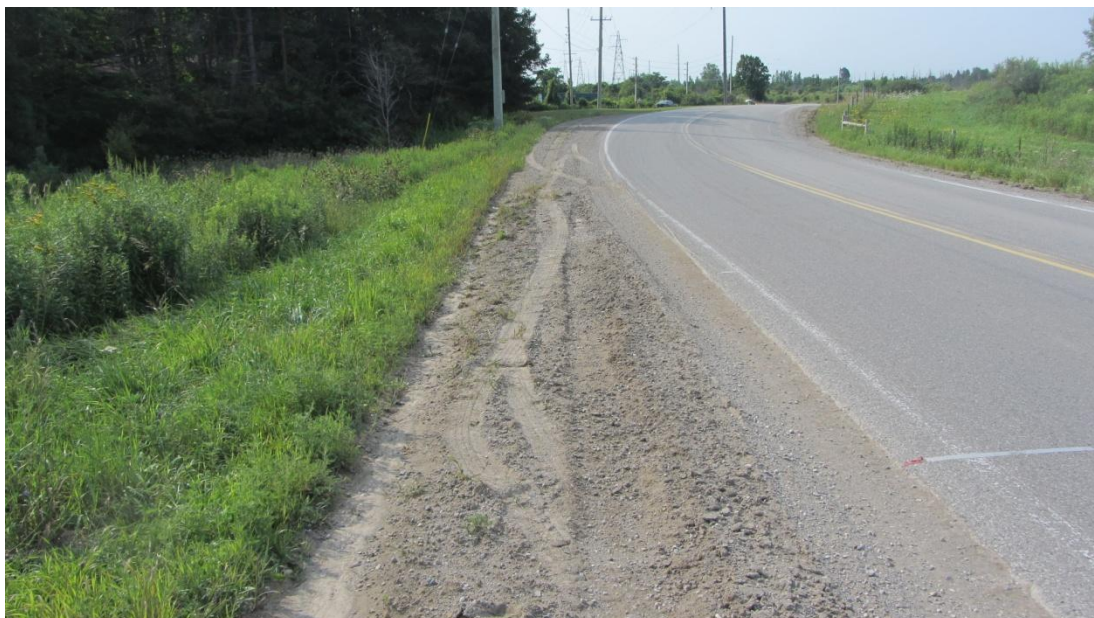
Figure 11: The driver makes a steering correction as evidenced by the separation in the travel path between the front and rear tires.
