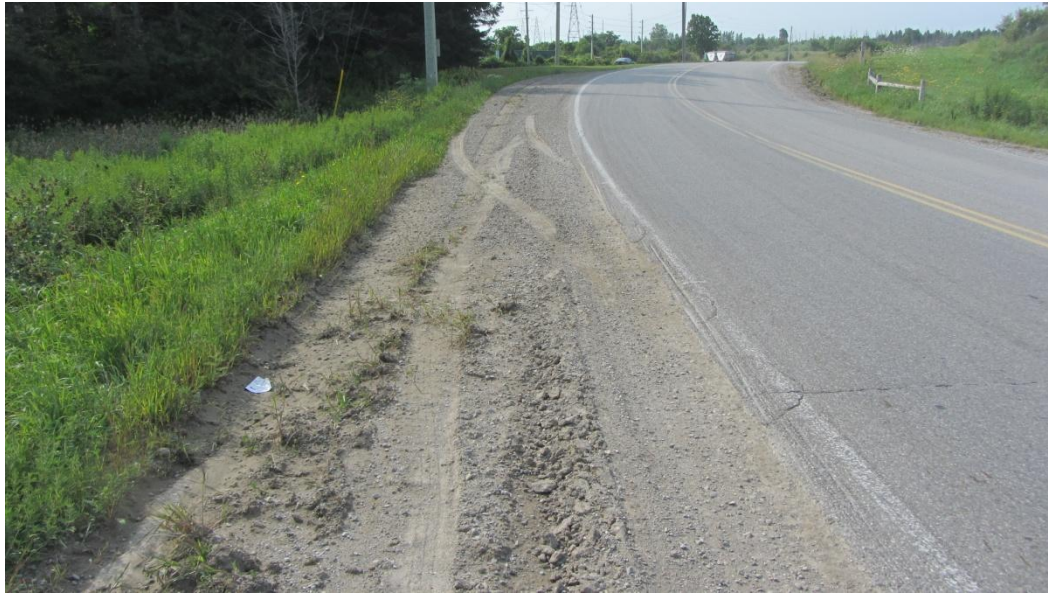
Figure 12: View of left side tires travelling in the middle of the shoulder while the right side tires are travelling in the grass roadside as the vehicle continues reversing.
